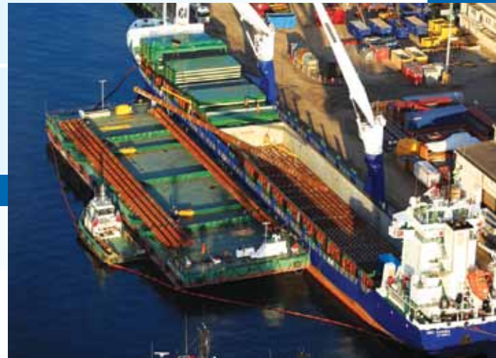
InterMoor uses a customized transport-and-launch barge to carry the conductors out to the site. This barge includes an InterMoor designed conductor side-launch system for keelhauling the conductors to the anchor-handling vessel (AHV). There are two (2) conductor shuttle systems on the barge. They are hydraulically powered and include several safety features.
