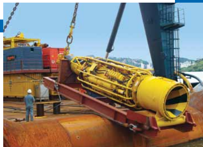
InterMoor uses MENCK's MHU-270T DWS which includes a deepwater hydraulic hammer, capable of providing a driving energy of 270 KJ at a water depth of 3,281 ft. (1000 m.) combined with MENCK's girdle-type electro-hydraulic power pack and umbilical support system.
