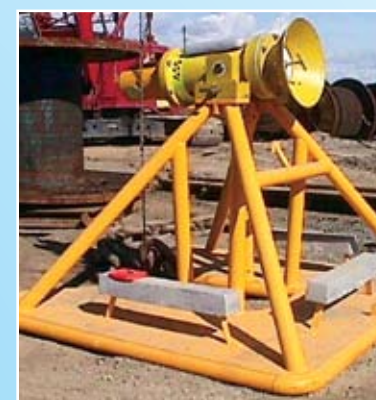
Specialized SEPLA installation equipment, such as this seabed connector, are fabricated at InterMoor's fabrication facilities.
